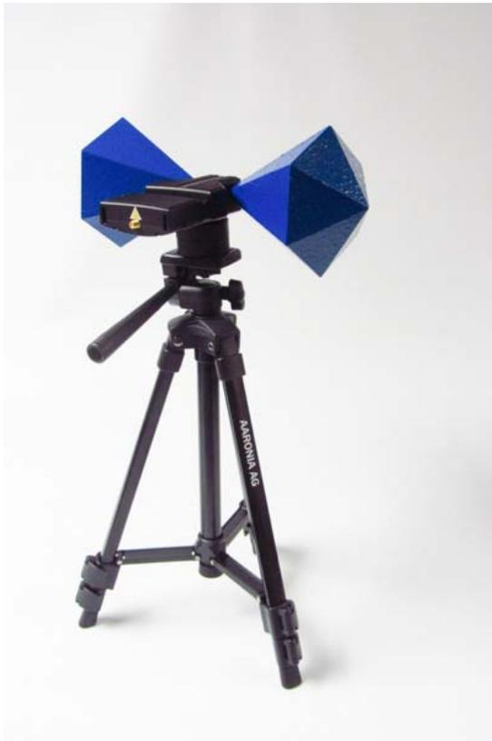
Figure 4 - The 30100X antenna mounted to the larger aluminum tripod, which may be extended to just over 1m in height. While perfect for these two antennas, the light weight design does not lend itself to larger EMI antennas.
