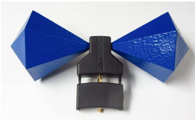
Figure 3 - The BicoLOG 30100X 30 to 1000 MHz biconical dipole active antenna with attached 40 dB gain preamplifier. The antenna connector is SMA.
