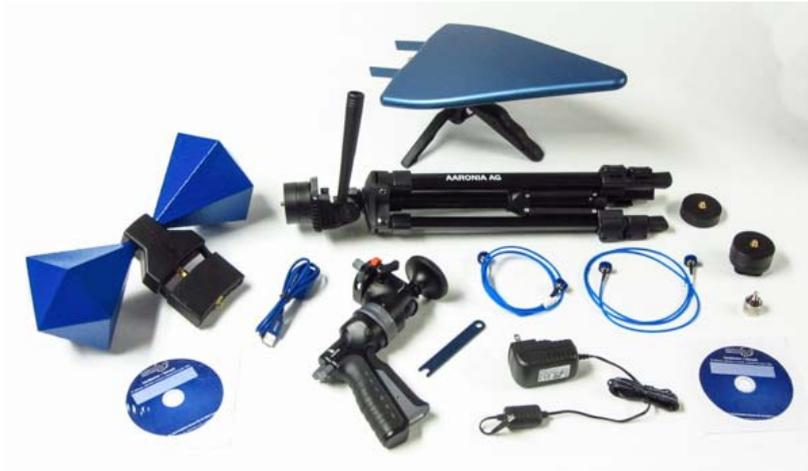
Figure 2 - The contents of the kit as received. The larger tripod and HyperLOG antenna were extras included for evaluation.
