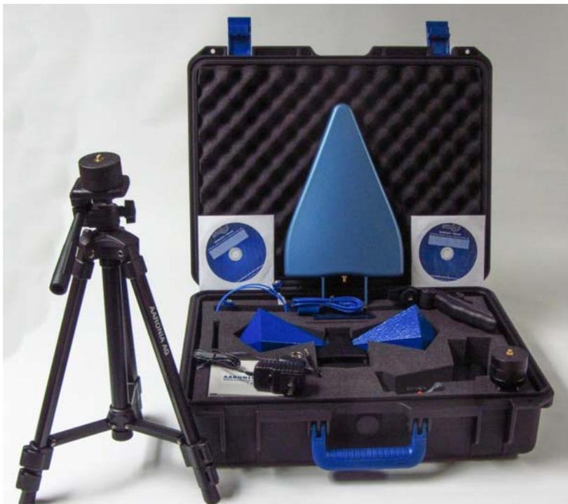
Figure 1 - The antenna kit as received includes the 30100X BicoLOG and HyperLOG 7060 antennas with all the accessories. The HyperLOG 7060 and larger tripod were optional extras, apart from the main kit for the BicoLOG antenna.
