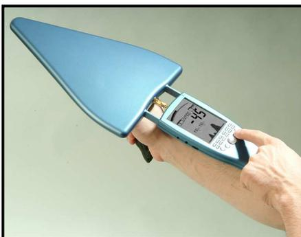
Using this method, you can **directly** attach the HyperLOG antenna to SPECTRAN for both to form a single, compact unit. This offers a few advantages for making adjustments during measurement, as keys can now be pressed all the time using your index finger. However, the HyperLOG antenna cannot be moved independently of SPECTRAN anymore, which might create difficulties in reading the display in cer-
