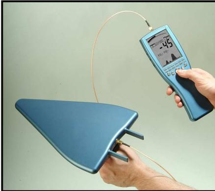
First, carefully screw the included **SMA cable** to the **SMA socket** on the SPECTRAN. The cable should be attached carefully. **Do not apply excessive force!** As soon as there is resistance, slightly tighten the plug using the **SMA tool**. Again, don't use excessive force. Never trigger the overtorque protection (the **SMA tool** has an overtorque protection and starts slipping as soon as **excessive force** is applied).
