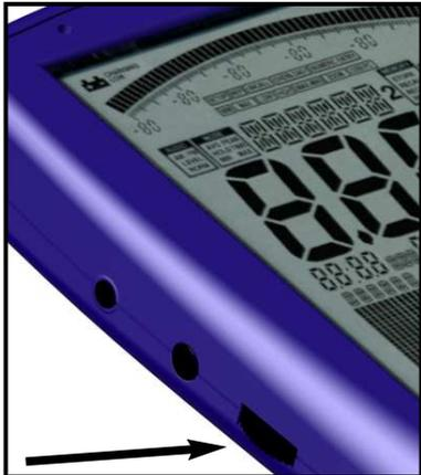
The Jog Dial, like on modern cell phones or PDAs, replaces the up/down arrowkeys (“turn” the jog dial) and the Enter key (briefly “press” the jog dial). Like this, you can e.g. control the complete menu system just with this handy little wheel.
