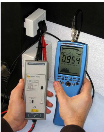
Measurement of a DSL line utilizing our Active differential probe.
