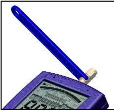
First, carefully screw the **SMA adapter** onto the **SMA socket** on the SPECTRAN. Screwing should be possible without much resistance. **Do not use excessive force!** As soon as you notice a resistance, slightly tighten the connection using the **SMA tool**. Again, do not apply excessive force! Never trigger the over-torque protection (the **SMA tool** features an over-torque protection as soon as **excessive force** is applied).
