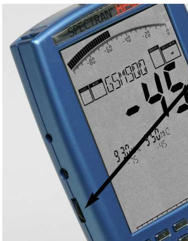
Volume can be adjusted with the volume control on the left.
