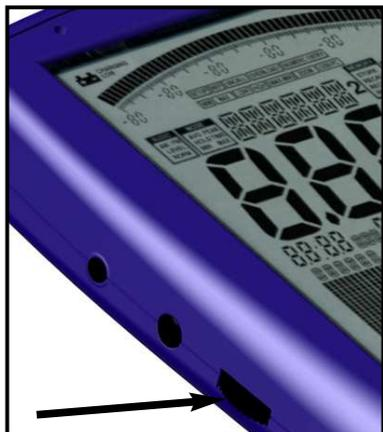
Using the **Jog dial**, you can activate a cursor in *spectrum analysis* mode. This cursor allows you to display the exact frequency and signal level of a certain point on the display. To activate the cursor, simply turn the Jog dial and the cursor appears as a line in the spectrum display. You can deactivate the cursor by pressing the menu key twice. The portion of the spectrum display under the cursor is drawn in inverse, so its information is preserved.
