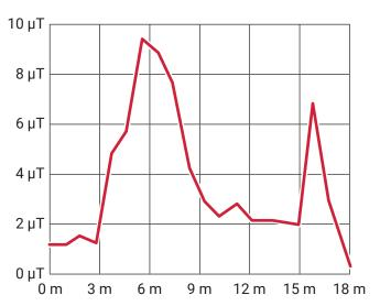
Transmission damping curves without MagnoShield DUR panel
