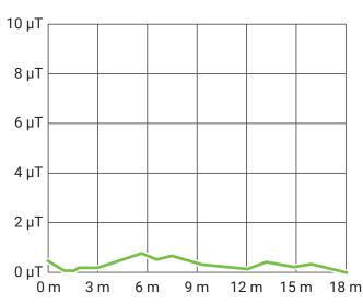
Transmission damping curves with MagnoShield DUR panel
