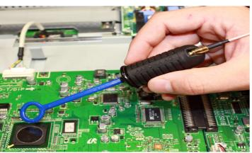
Pinpointing interference sources on a circuit board
