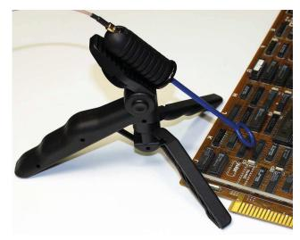
Pinpointing interference sources on a circuit board
