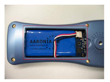
To open the battery compartment you will need an ordinary screwdriver. Loosen the screw on the battery compartment cover until this can be removed easily.
