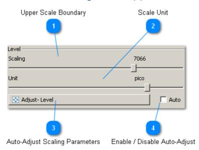
If the view uses a non-decibel based <u>Display Unit</u> the <u>default level controls</u> will be replaced with an alternate set of scaling controls. Switching back to a decibel based Display Unit will also switch the controls back.
