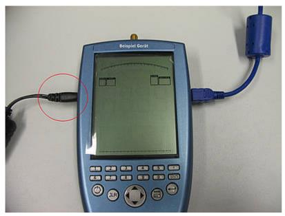
Connect the SPECTRAN via USB cable to the PC. Then connect the charger / power supply to make sure that your SPECTRAN can be turned on.
