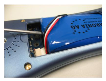
Unplug the charger from the SPECTRAN first. To disconnect the battery in the device, it must be lifted carefully with a screwdriver. It is important that the front edge of the battery is over the plug. So it is possible to pull the plug backward under the battery in the next step.
