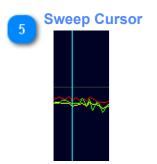
Visual aid that shows where the device is currently sweeping. Can be enabled / disabled in the Spectrum Control.
