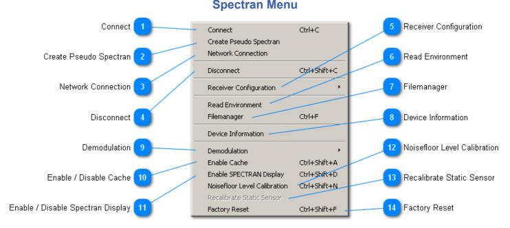
This menu contains device related actions for connection management and controlling advanced features. Note that some actions may not be available, either because the device doesn't support the feature or because the action isn't valid for current device or software mode.
