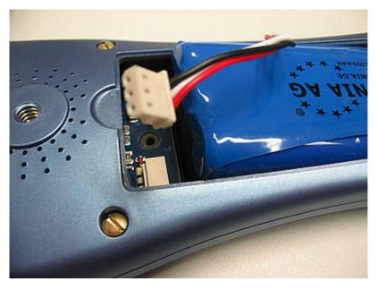
Hold with one hand the raised battery. Now take the screwdriver and push the plug from the socket under the battery. If the plug is completely disconnected from the socket, the cable can be attached on to the battery.
