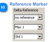
Select a Reference Marker that will be used as base for displaying measurement and frequency offsets in the <u>Spectrum View</u> and <u>Marker Legend</u>.
