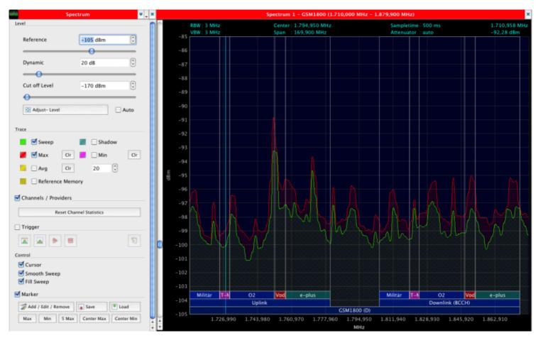
In the <u>Spectrum Control</u> you can adjust the <u>Reference level</u> and <u>Dynamic range</u>, or just use the <u>Adjust-Level</u> button to let the MCS determine suitable values automatically. Changing the Reference level simply moves the graph up or down, while the Dynamic range determines the vertical resolution of the graph. Measurement values below the <u>Cut off Level</u> are discarded, this way you can remove noise from the graph.
