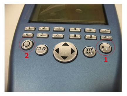
To start the emergency program, simultaneously press the "ENTER" and "ON" button. The SPECTRAN now starts an emergency program and logs on to the PC. Please note that during the emergency program there is no indicator on the display!
