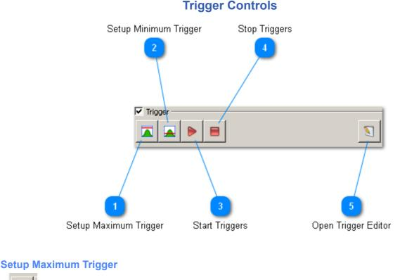
Set up the default maximum trigger. For further information see Measurement Triggers.
