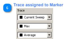
Each Marker can be assigned to a specific trace in the Spectrum. For example you can add a Dynamic Maximum Marker to both the Current Sweep and the Maximum trace to keep track of the current and the absolute maximum of a measurement. Note that not all traces are available for marker assignments.
