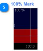
When the <u>selected scaling</u> exceeds 100% a reference marker is shown at the 100% position.
