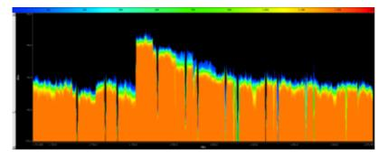
Filled Mode: Like Lines Mode, but also updates all points between the line and the reference level Changing the Display Mode will cause a <u>reset</u> of the view.
