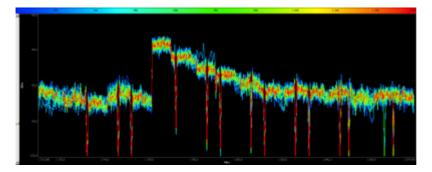
Lines Mode: Calculates a line between subsequent points and updates all points on this line.
